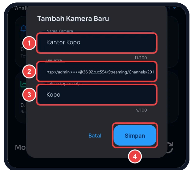
Example: Hikvision DVR, camera on channel 2 (password & IP masked)
